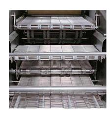
Our optional triple-flip conveyor for hard-to-coat products can easily convert to a straight-through conveyor.
