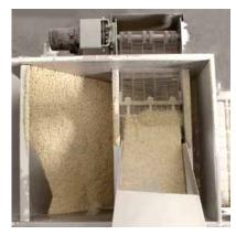
Sifter conveyor removes lumps from non free-flowing breading hopper.
